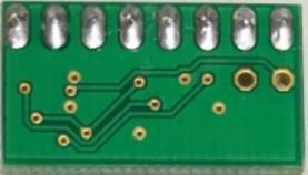
8-pin-header assembled and soldered to top-side of the USB-module
